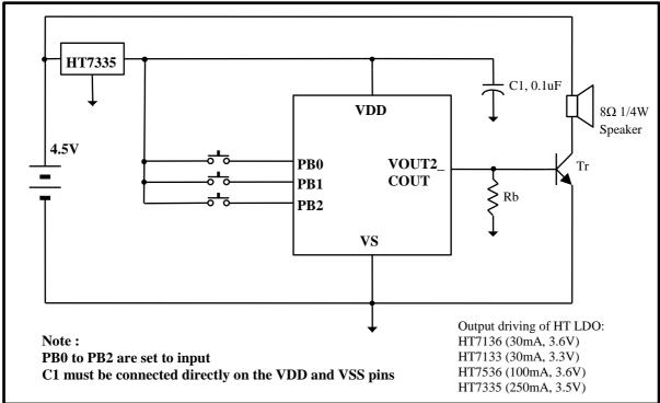
Using 4.5V Battery with COUT speaker drive
