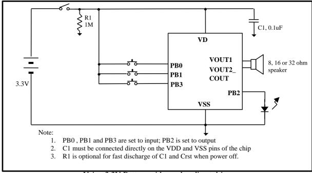
Using 3.3V Battery with speaker direct drive
